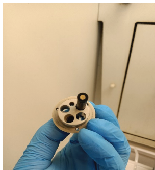
Figure S2.8. Au voltammetry electrode before (a) and after (b) voltammetry experiments under CO 2 purging with Ag as the counter electrode. The deposition of silver is visibly observed after the voltammetry experiments. The supporting electrolyte used was 0.5 mol% MM NTF 2 .
