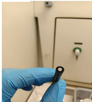
Figure S2.8. Au voltammetry electrode before (a) and after (b) voltammetry experiments under CO 2 purging with Ag as the counter electrode. The deposition of silver is visibly observed after the voltammetry experiments. The supporting electrolyte used was 0.5 mol% MM NTF 2 .
