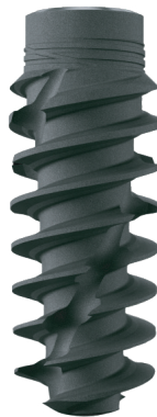
Figure 3. Straumann BLX implant RB. Roxolid® implant material with SLActive® surface. Full tapered core with bi-directional cutting threads, chipflute for redistribution of bone chips, microthreads on the implant neck to reduce stress at cortical bone. Conical implant abutment connection (TorcFit™). Courtesy of Straumann AG.
