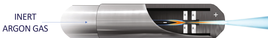
Figure 3 PlasmaJet device: argon gas is heated to generate plasma. (-) Cathode; (+) Anode; (IE) Intermediate Electrodes.
