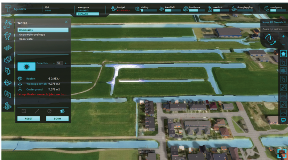
Fig. 5.2. Impression of the user interface of RE:PEAT. All users see the 3D simulation from their own perspective. The left bar contains possible actions, the right bar contains thematic maps, the top bar contains drop-down panels with information on goals, budgets, and a comparison of results with and without actions.
