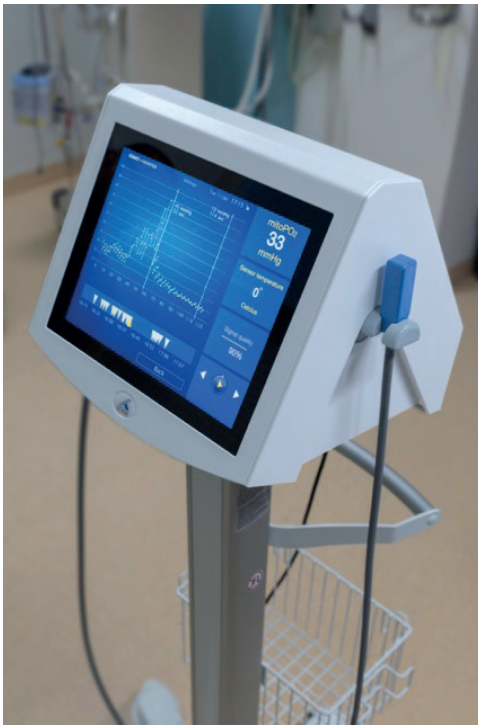
Fig.1 COMET monitor and skin sensor.
