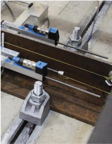
**Figure 2.10** | Pretensioned channel connector [134, 135].
