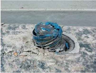
(a) Coupler with part of fractured bolt.
