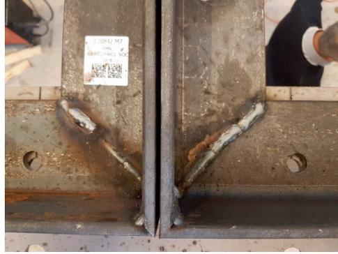
(b) Detail of angle profiles at midspan.
