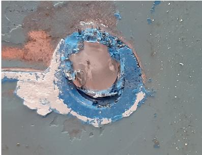
(c) Embedment of steel-reinforced resin due to reduction of confinement effects.
